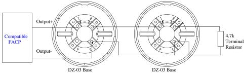
CAUTION: DO NOT USE LOOPED WIRE UNDER TERMINAL 3. BREAK WIRE RUN TO PROVIDE SUPERVISION OF CONNECTIONS.
