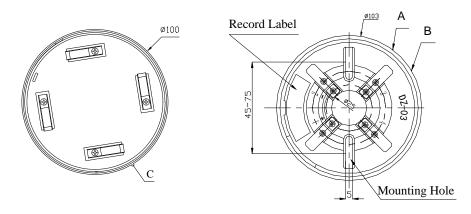
Fig. 3 Bottom of the detector
